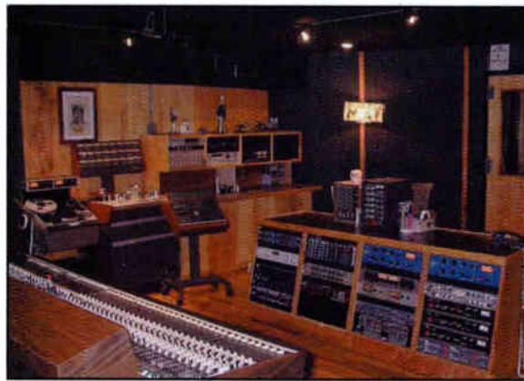
Coyote Recording Studio's control room boasts an API console, Studer multitrack and Pro Tools with Pro Control.
