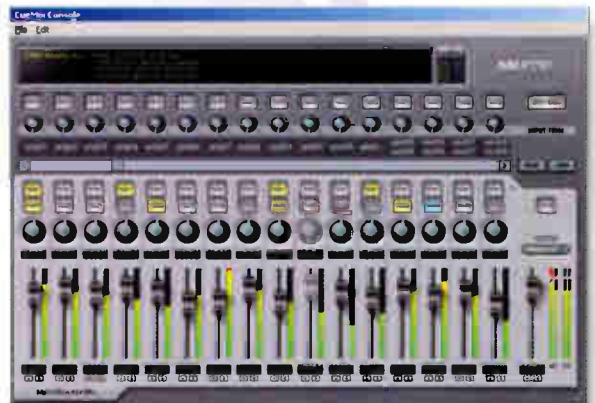
Our cross-platform CueMix Console works side by side with your audio software to give you a no-latency mix bus for every stereo output in your PCI-424 system.
