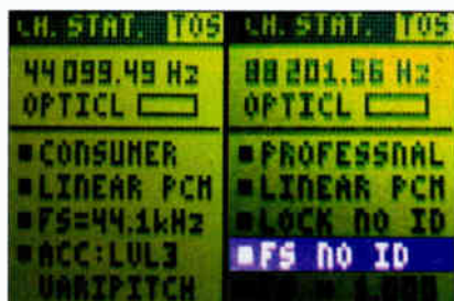
Fig. 1: Channel-status display comparing outputs of a Technics CD player (left) and an early Alesis MasterLink.
