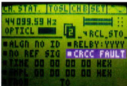
Fig. 2: The three channel-status pages alternately flash "CRCC ok" and "CRCC Fault" (shown in reverse video for clarity) to indicate a problem. Note: The black rectangle next to optical also indicates a data problem that was not severe enough to mute audio.
