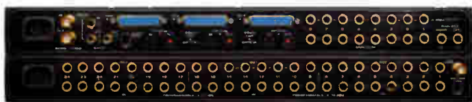
Together, a 2408mk3 and 24I/O give you 32 analog and 24 ADAT/TDFIF digital inputs and outputs in a compact, affordable system.
