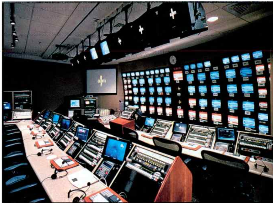
The main control room at Times Square Studios Ltd., with 15 user stations, is centered around a 256-port CS9600 RTS ADAM Matrix System from Telex.
