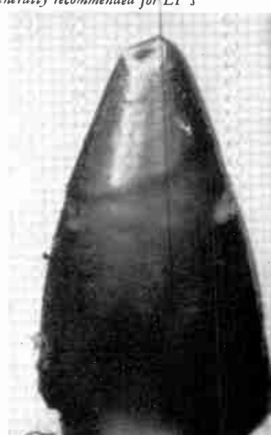
Microphotos of styli. Left to right: 1. Perfect diamond stylus. 2. A sapphire stylus starts to wear down quickly. 3. When a sapphire wears to this extent, it will destroy an LP in one playing. 4. Osmium wears so quickly it is not generally recommended for LP's
