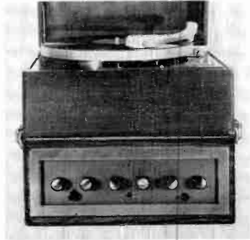
Fig. 3. You may prefer this arrangement of the preamp-amplifier and a Presto turntable, with the two wood cases fastened together
