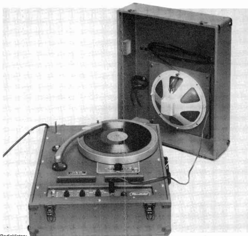
Fig. 1. This portable Rek-O-Kut instrument has additional connections for a radio and a microphone to be used with the built-in loudspeaker
