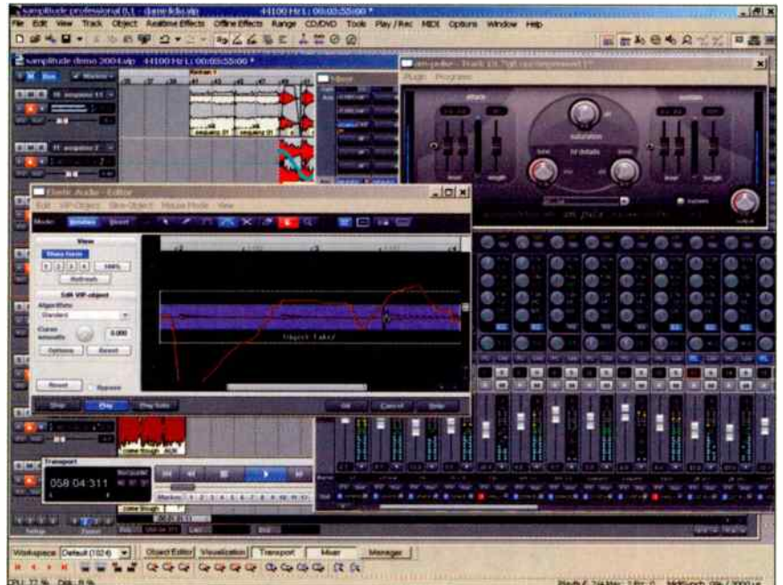
Fig. 1. Samplitude 8's elastic audio feature offers multiple ways to use the process, covering the range from subtle pitch correction to extreme effects.
