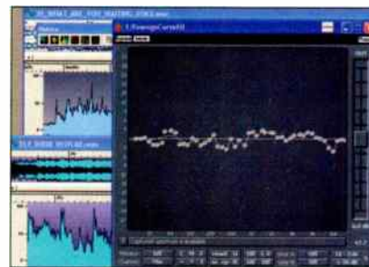
Fig. 3: Voxengo's CurveEQ has analyzed the song in the rear window, matched it to the current song in the front window, and generated a compensating response curve so that the current song's spectrum matches the reference. This curve can be tweaked further.
