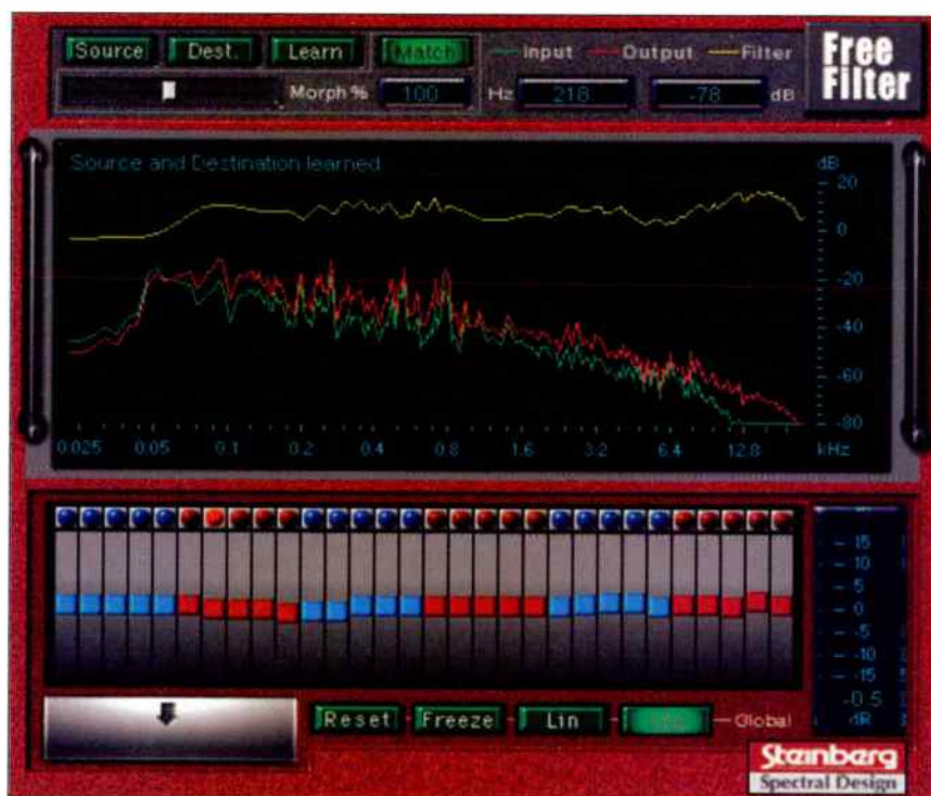
Fig. 2: Steinberg's FreeFilter was an early curve-stealing/EQ program. Its sound quality is lacking by today's standards, but its functionality set the paradigm for this type of software.
