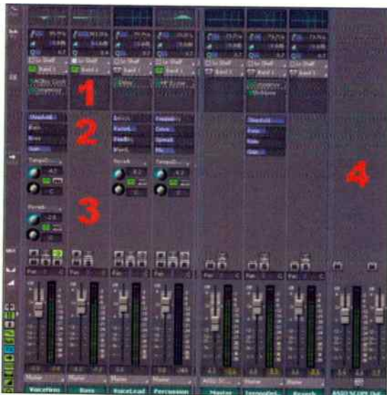
Fig 4: Just below a channel or bus EQ section in Sonar 4 Producer Edition, you’ll see the effects bin (1). Below that are four realtime controls for effects parameters (2), then the send controls (3). All insert effects are pre-fader, but all sends can choose between pre and post. Note that the hardware out on the right (4) has no effects slot, because master effects are handled through a master bus.
