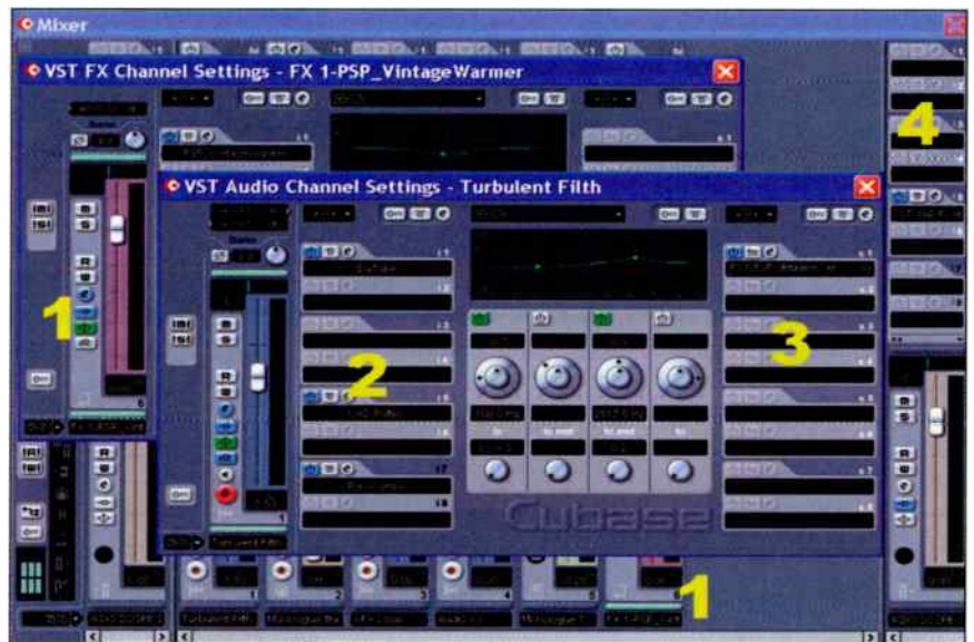
Fig. 1: With Steinberg's Cubase SX3, insert, send, and master effects all have six pre-fader and two post-fader slots, and look similar. Send effects go in a separate FX track (1), which returns to the mixer. Individual channels have inserts (2), as well as eight send controls (3). The master outs (4) have a similar structure.
