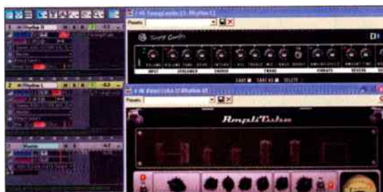
Fig. 1: Native Instruments' Twang Combo and IK Multimedia's AmpliTube 2 are being treated like a guitar setup that splits into two different amps. Each plug-in is inserted into its own track, but fed by the same guitar signal.
