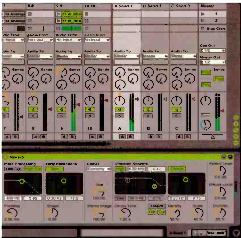
Fig. 3: Ableton Live's Reverb has been inserted into the A Send 1 bus, thus saving considerable CPU power over inserting several instances into multiple tracks.
