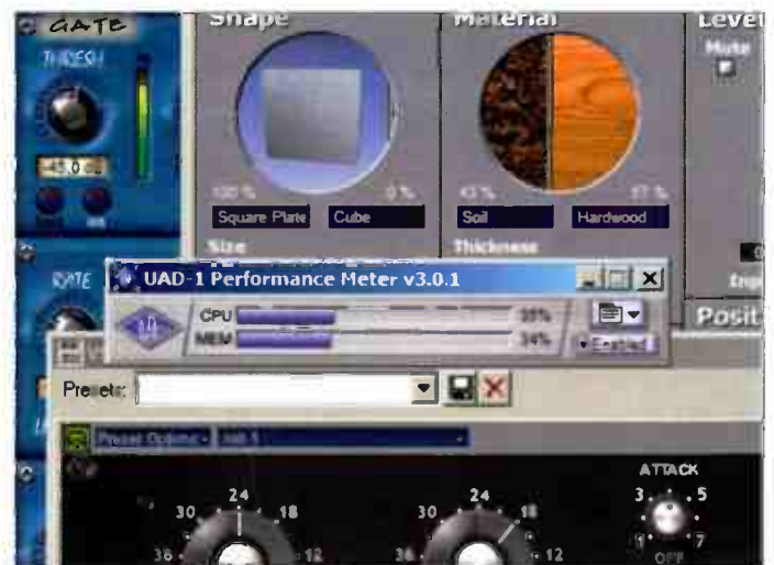
Fig. 2: Even running a reverb, heavy-duty guitar amp simulator, and limiter, the UAD-1 is using only 35% of its onboard CPU's capacity.
