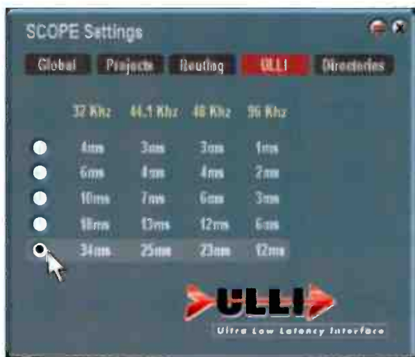
Fig. 1: When mixing, 20 or 30ms or latency will let you run more plug-ins, with a negligible tradeoff in performance.
