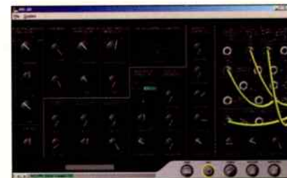
The patch cords toward the right of this screenshot were patched not in software, but by using a physical hardware controller.
