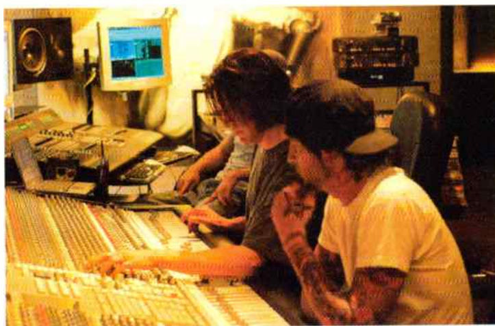
Scott Humphrey and Tommy Lee at the Chop Shop's SSL 4000 G+ console. External mic preamps were used for tracking Lee's drums to an Ampex 2-inch analog recorder.
