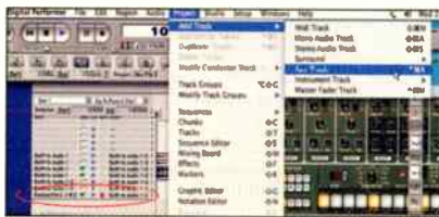
Assigning a client output to the Input field in an Aux track (circled in red) feeds the output into Digital Performer's mixer.
