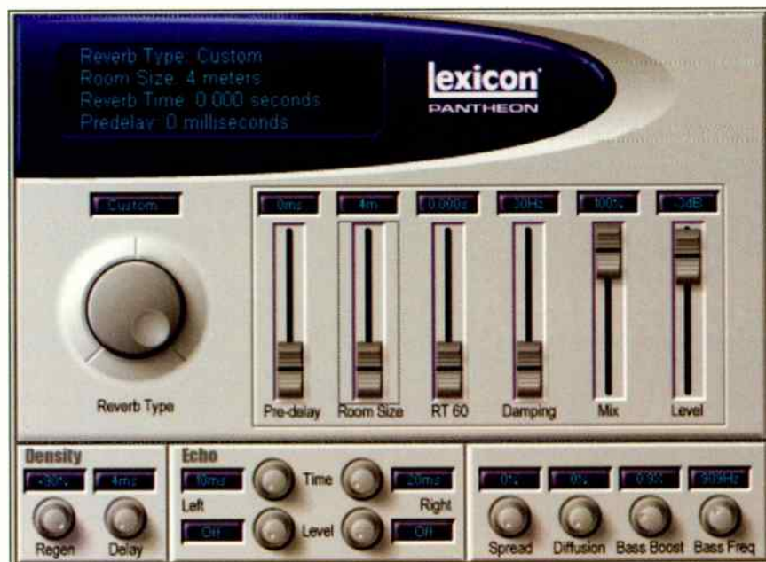
It says it's a reverb, but here Pantheon is set up as a resonator.
