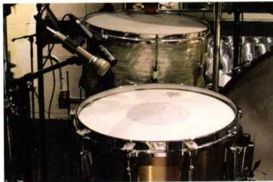
Two mics were positioned above the snare drum, and a third was positioned below. The mic below was gated to cut down on leakage.
