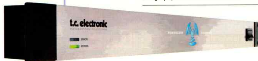
PowerCore FireWire fits in a slim, 1U box, but contains a lot of hardware DSP power.
