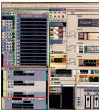
Cubase's Storm 3 device panel (outlined in green) is toward the upper right; three channel pairs are active. The connections window patches the Storm instruments to various ReWire outs. The lower left shows the ReWire channels (outlined in red), and directly below, a MIDI track driving one of the instruments.
