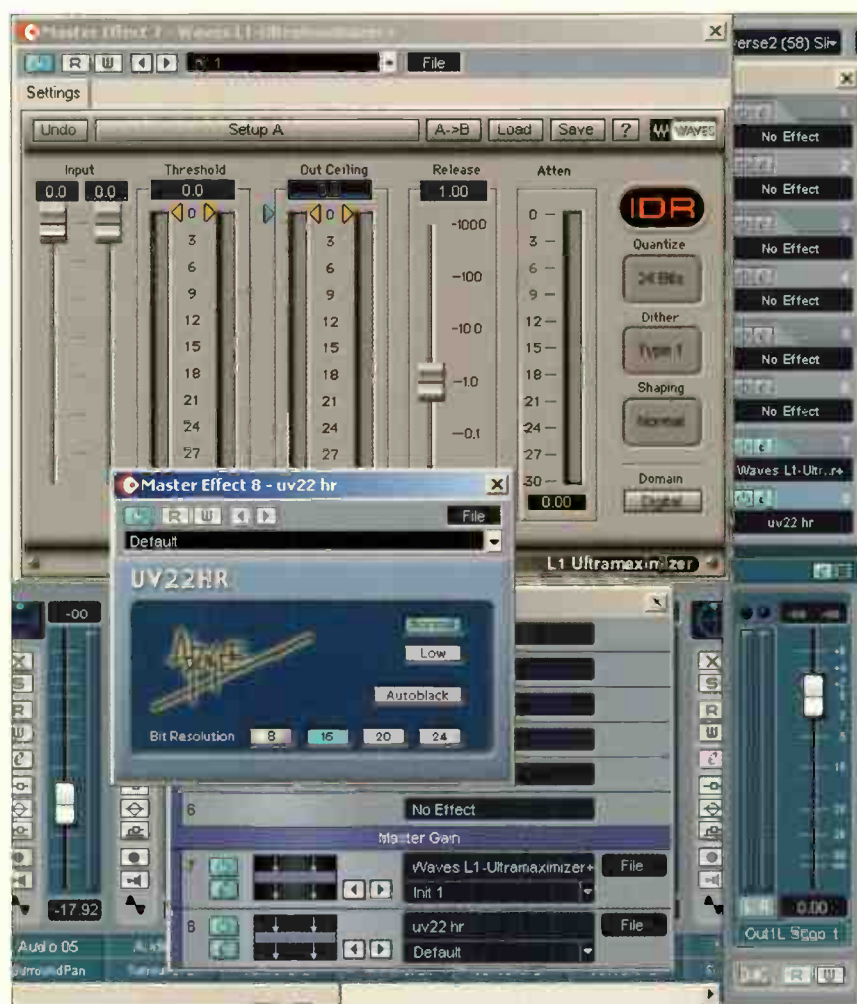
Fig. 1. Cubase includes dithering that defaults to being enabled, so if you use this, make sure that any other master effects plug-ins you add don't have dithering enabled. Or, disable Cubase's dithering section and use the other plug-in's dithering instead
