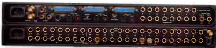
Together, a 2408mk3 and 24 I/O give you 32 analog and 24 ADAT/TDIF digital inputs and outputs in a compact, affordable system.
