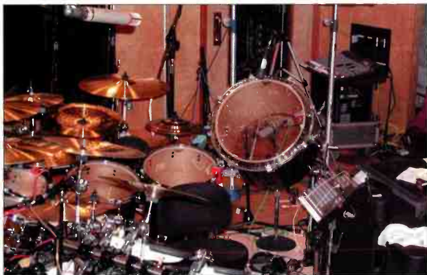
David Silveria's amply miked kit. Shown here: the four overhead mics and snare drum mics.
