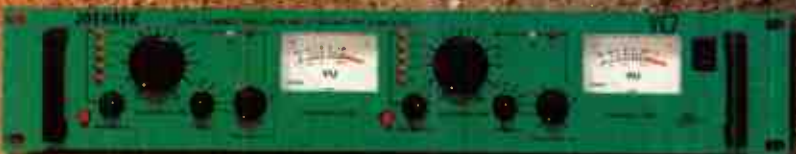
VC7 Dual Channel Mic-Pre with impedance matching & selectable Hi-Pass filters $1,299.99
