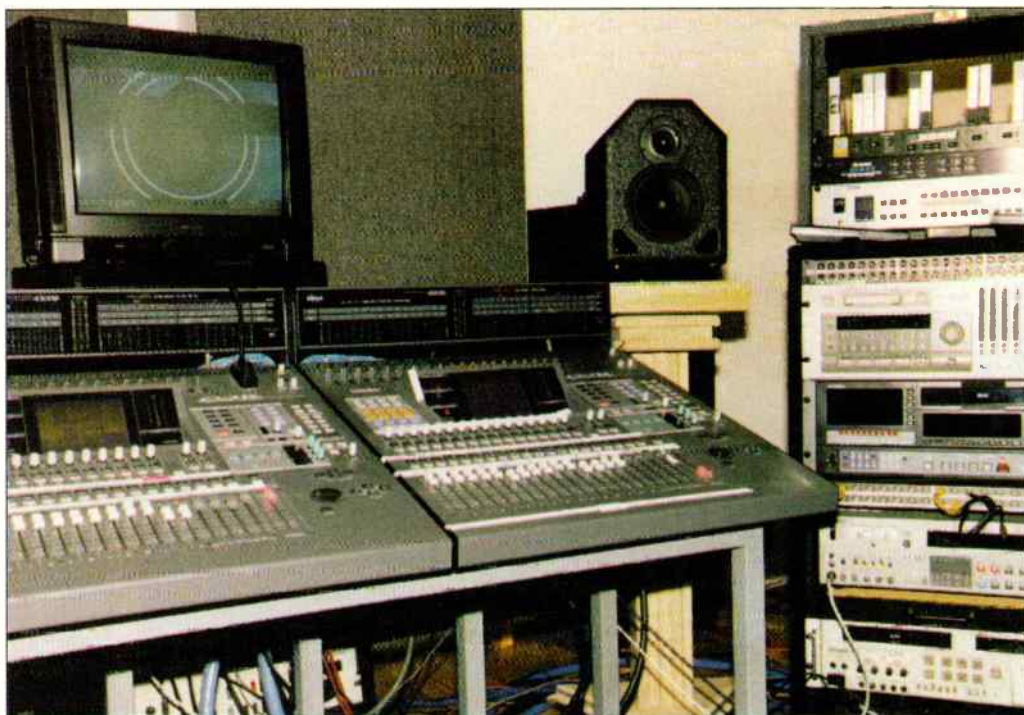
MULTI-TASKER: The total recall feature in Haslinger's two Yamaha 02R digital consoles allows him to work on several projects at once.
