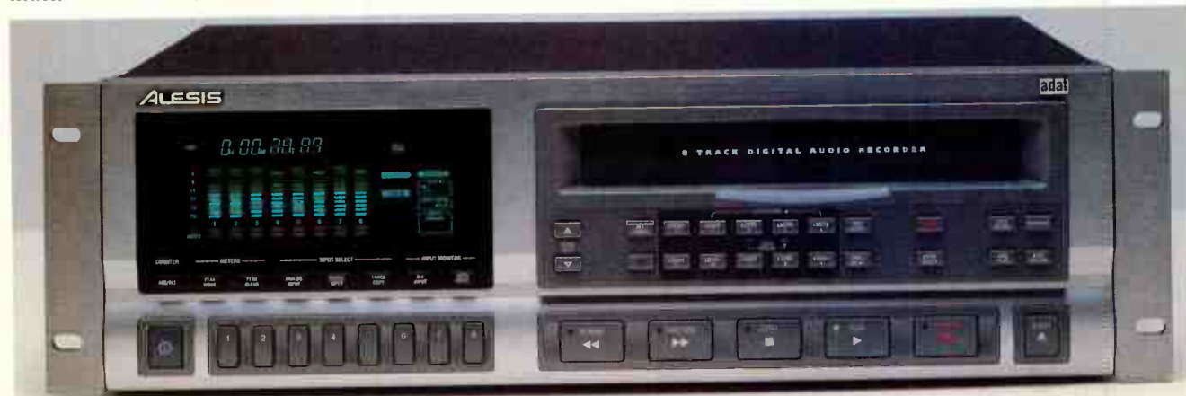
ADVANCED ADAT: Among the improvements that the Alesis ADAT-XT offers are faster and more accurate transport controls and on-board editing.
