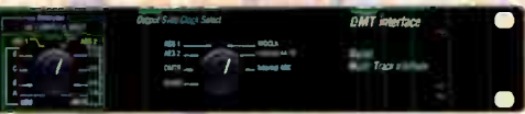
The DMTi option for direct digital connection to the Alesis ADAT ® and Tascam ® DA88.
