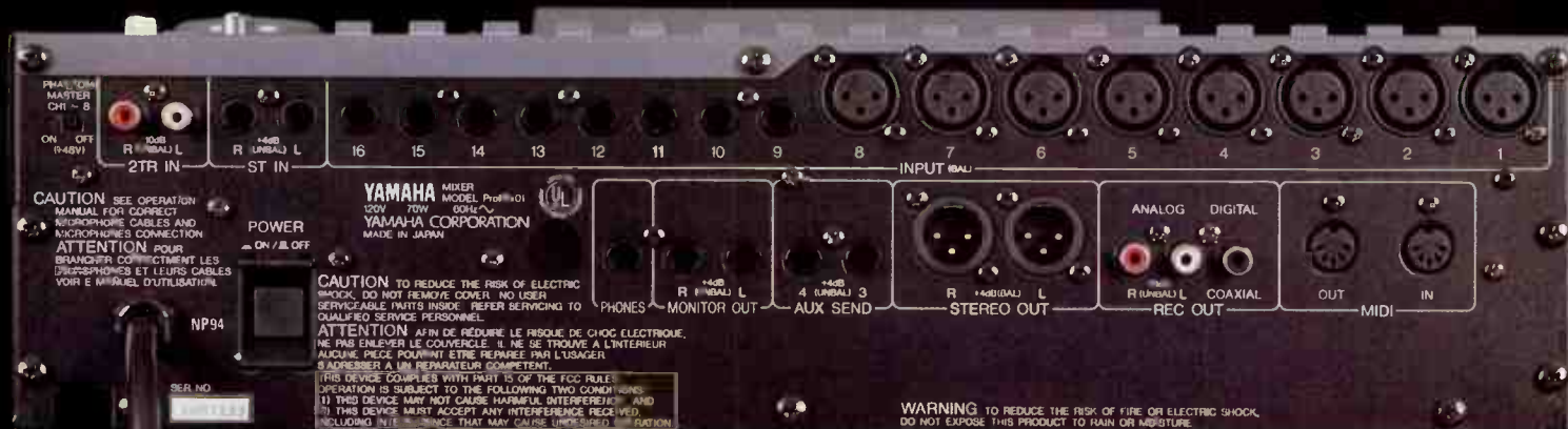
WELL CONNECTED: The ProMix 01 has lots of inputs, but no digital ones.
