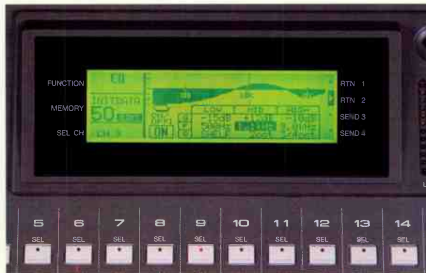
EQUAL TIME: The ProMix 01 has 30 preset EQ programs and space for 20 user programs.
