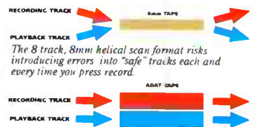
The ADAT format records each track discretely, as all professional multitrack recorders should.
