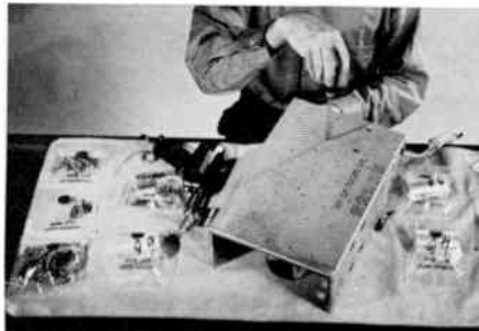
The cloth makes an excellent work surface since small bits of hardware and tiny electronic parts won't roll or slide off it. Tricky-to-wire parts of the circuitry come pre-assembled on plug-in printed-circuit boards.
