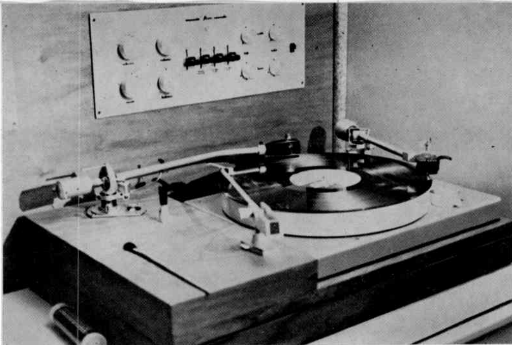
Multiple tone arms mounted on a turntable sets the stage for stereo phono cartridge comparison tests.
