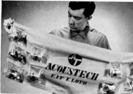
Components and hardware are packaged in numbered plastic bags (like one shown above) that are stapled to a fuzzy-surfaced, solder-resistant cloth. You open one bag at a time to carry out a group of instructions.
