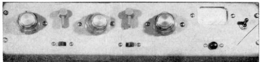
Controls, left to right: dual record gain, input 2, equalization lever, output switch, dual record gain, input 1, record selection lever (upper track, lower track, stereo) meter selection switch, dual playback gain, meter with zero set, and on/off switch.
