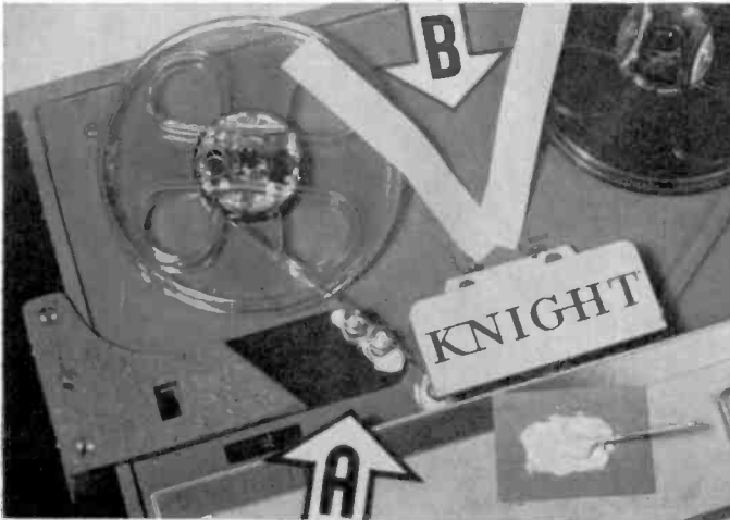
Upper left: Fig. 6—The "Sensor Unit" consists chiefly of two metal TAPE GUIDE POSTS firmly epoxy-fastened to a wooden "jig" that holds them in proper place on the tape deck of my recorder. When a strip of metal foil, which is on the rear of the recording tape, comes by, it "joins" the posts, making the electrical contact that works the relay. Upper right: Fig. 7—Tape guide posts come in various shapes and sizes. The Nortronics pair ("A") that I used are large enough to make working with them quite easy. For more compactness (especially if this is to be a permanent addition to your tape deck), SONY has some very small guides ("B"), or you can make your own out of phone tips ("C"). Lower left: Fig. 8—Keep in mind, when picking out a spot on your tape deck ("A") for locating the two Guide Posts, that it is the BACK of the recording tape that must come in contact with the two guides. Also, if you limit yourself to using a 5" reel when making narration tapes, this will give you a lot more room for placing the Sensor Unit. Lower right: Fig. 9—Epoxy adhesive securely anchors the guide posts in place . . . then the two wires are soldered on afterwards. Underneath each guide post (though not visible here) is a metal washer that lifts the post up just exactly high enough for accurate tape travel. Note the FOIL STRIP about to make contact with the two metal posts.
