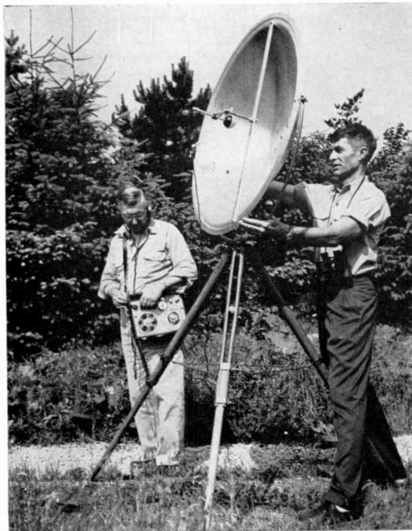
The author (right), and Dr. Carl R. Reese, a colleague, capture a bird's melody with a Magnemite portable, and microphone mounted in a 40 inch parabolic reflector. The parabolic is aimed by sighting through a small hole near the center.
