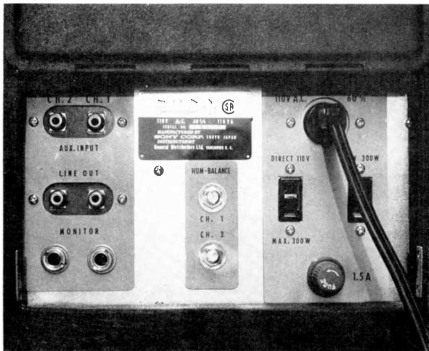
The Sony 521 has an AUX. INPUT to take a high level signal from a phono preamp for recording purposes and the LINE OUT sockets would feed an AUX. input on the same preamp for playback purposes. An added feature of this machine is a pair of MONITOR sockets so that the owner can use stereo headphones or external speakers for monitoring during an outside recording session.
