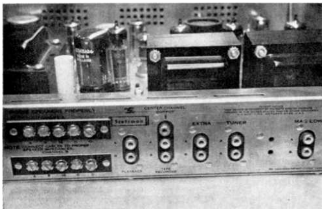
On this H. H. Scott integrated preamp/amplifier the PLAYBACK sockets (marked "A" and "B" for the two stereo channels) accept the outputs of tape heads direct and the TAPE RECORDER sockets feed a high level signal to the two respective RADIO inputs, or the HI-LEVEL inputs of a tape deck amplifier. AMPLIFIER outputs of a complete recorder could be fed either into the EXTRA or TUNER inputs on this particular piece of equipment.
