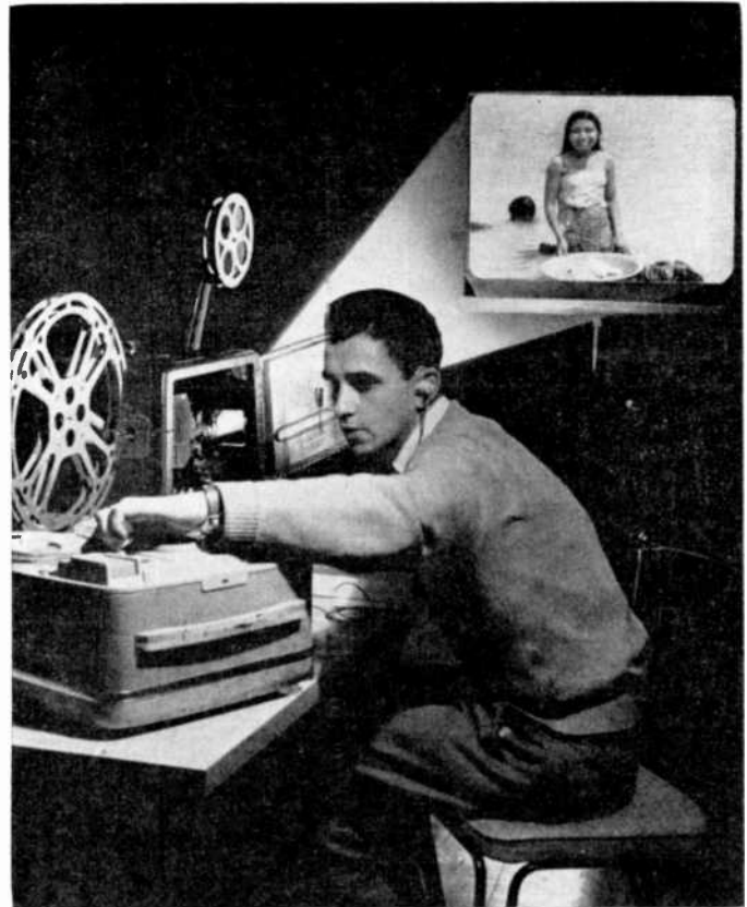
The author uses a Bell & Howell 302 magnetic projector to rerecord from a Revere tape recorder. The tape is kept in synchronization with the instant start-stop button. Note earphone for monitoring.
