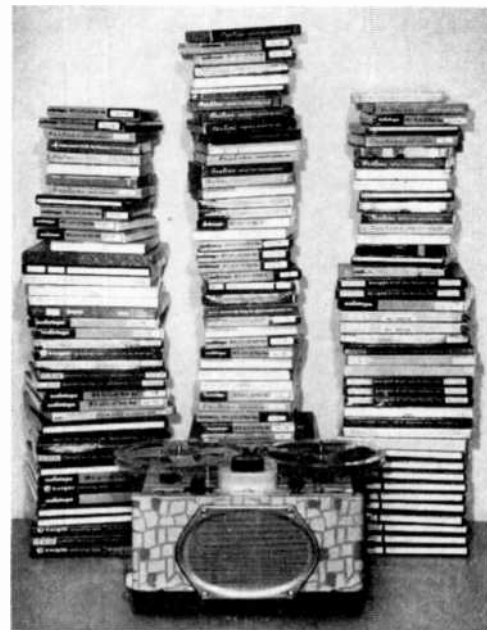
Fig. 2: Imagine the money saved by using three-fourths of this tape over again. Here is a precious personal collection of monaural, twin-track tapes recorded at 7½ ips. A new recorder can re-record these onto four tracks at 3¾ ips with very little loss in quality, "condensing" everything down to a mere one-fourth in space.
