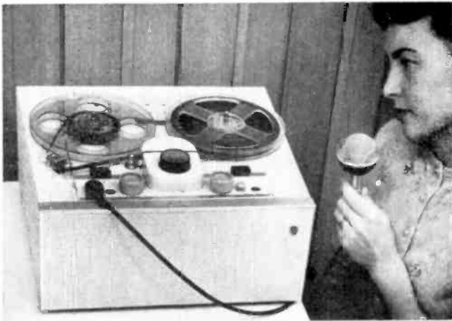
Fig. 10: The "Echo Master" ready for action. Or, if you'd rather have a Stereo Tape Editor instead, then use a similar unit arrangement but with a stereo play head in your auxiliary assembly. And "pipe" both stereo tracks through the recorder's single speaker, which will be plenty adequate for monitoring the tape while editing.
