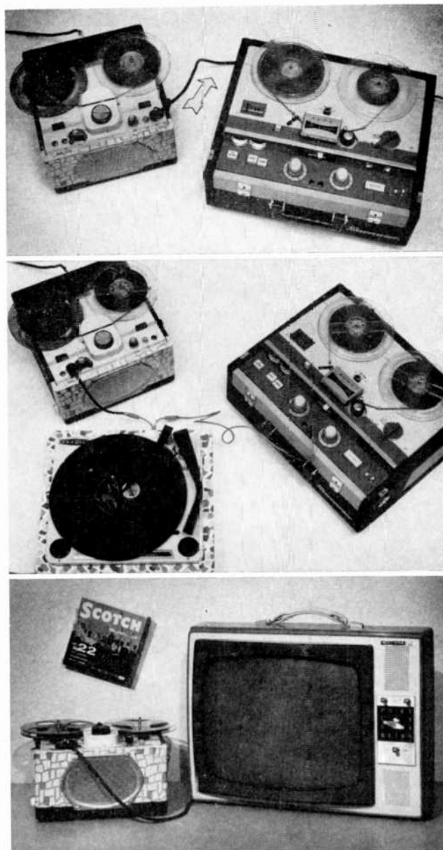
Fig. 3, top: To re-record (copy) a tape, plug the output of one recorder into the input of the other. This makes tape editing a simple and pleasurable task. When copying, the new tape can be balanced in volume, deletions can be made where wanted, and various selections can even be "reshuffled."
