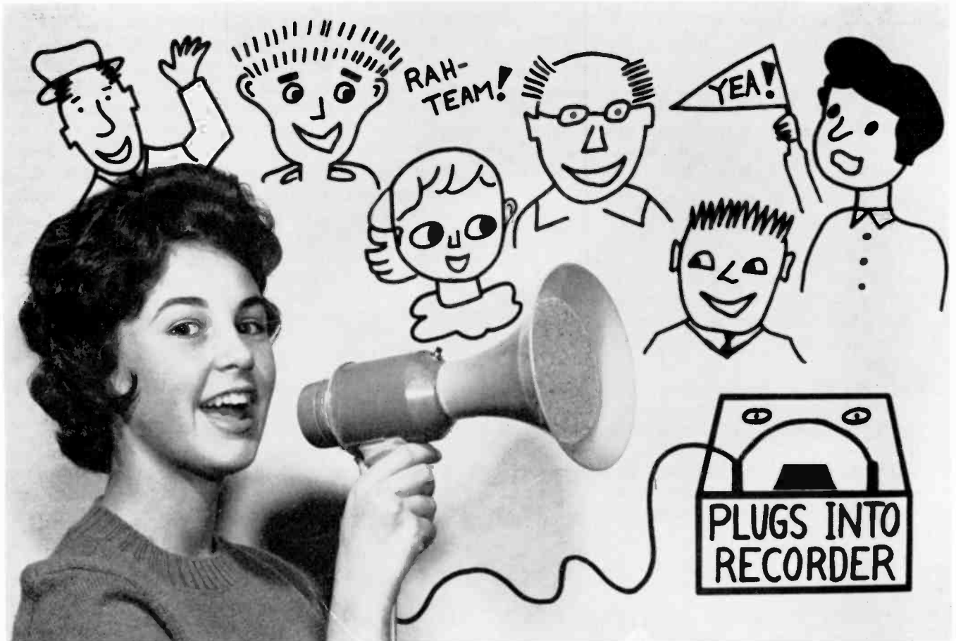
Fig. 1: "Yea, team!" Whether you're rooting for the home basketball squad or simply leading a group of squaredancers, this highly efficient Sound Gun—which is plugged into your tape recorder for power—comes in handy to amplify your normal voice to a loud roar.
