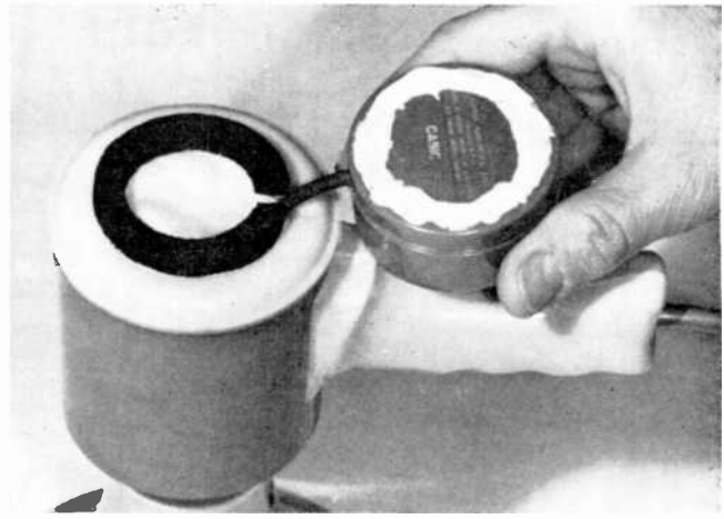
Fig. 10: A 1/4"-thick rubber "gasket" is first Epoxy-fastened to the rear of the Sound Gun, around the previously cut-out hole made for wiring ease. Then the rear chamber is completely, solidly packed with cotton, to keep the speaker vibrations from affecting the microphone, which here is all ready to be "Epoxyed" in place.
