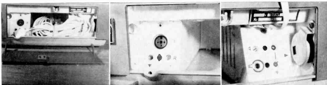
Removable door in side of case covers storage compartment and inputs and outputs. Left: cords and mike fit in center wall. Center: PA amplifier switch is metal button at upper left of photo. Grouped on panel are microphone jack, radio-phono input jack and output jack for playing through separate amplifier. Right: other panel contains headphone jack, external jack and voltage adaptor (with small window).
