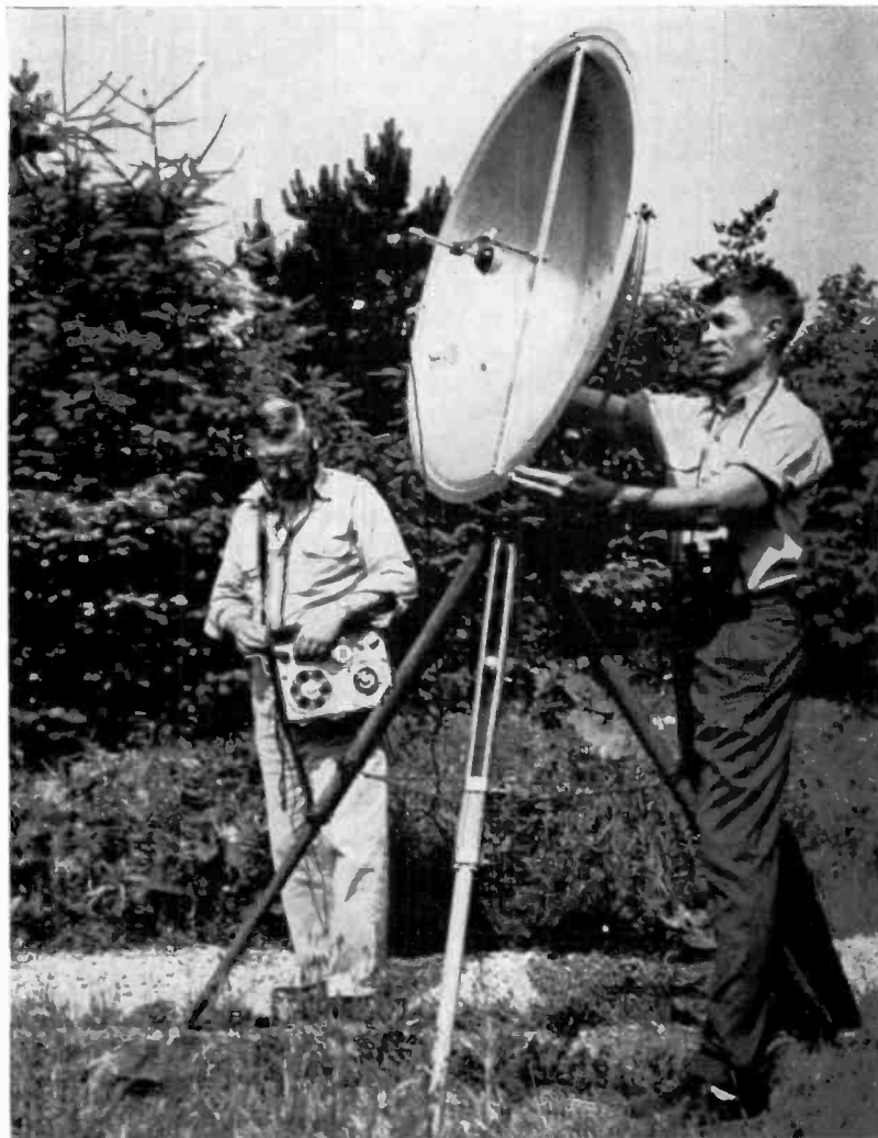
Recordists working in the field away from power sources, capture a bird's melody with a Magnemite portable, and microphone mounted in a 40 inch parabolic reflector. The parabola is aimed by sighting through a small hole near the center.
