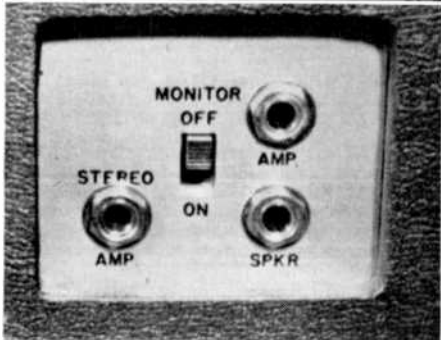
Upper left: Lid has holders for microphone, line cord and stereo connection cord. Upper right: the head covers are easily removed giving quick access for cleaning and demagnetizing. Lower left: output panel which has jacks for stereo amplifier, external speaker and external amplifier plus monitor switch. Lower right: inputs are for microphone and radio/phono.
