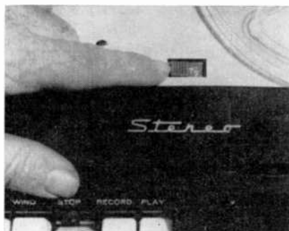
Speed change between 3¾ ips and 7½ ips is effected by moving the switch situated between the reels.
