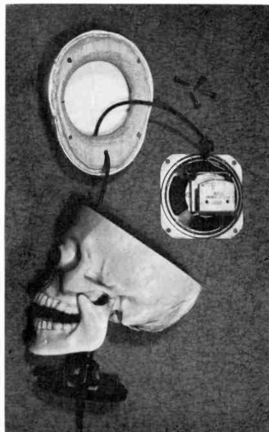
The manner in which you fasten the speaker is quite important. Experiment a bit to find the most suitable way. Here, a piece of wood is glued into the "cap" of the skull, then the speaker is fitted in place and fastened tight with wood screws. With this mounting, a hollow "spooky" sound is produced by the speaker.
