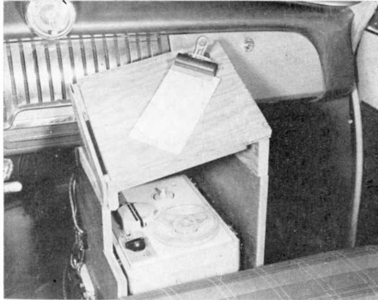
Fig. 1: Recorder installed in front of car within easy reach of driver makes learning while you drive easy. Inverted to supply current may be mounted ahead of firewall or in trunk of car to supply 110 volt current.
