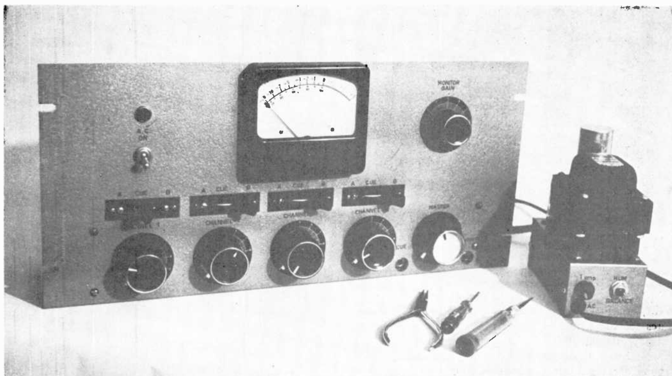
Wide spacing of controls on a large front panel gives ease of operation and eliminates possibility of knocking off controls in error. Large meter is easily seen.
