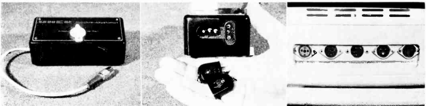
The Akustomat is an accessory which permits the recorder to be voice operated, turning itself on when the first words are spoken and stopping when the voice stops. It will also record supersonic signals on the tape for slide projector operation. It is shown at left. Center, plugs are furnished to connect to slide projector for automatic operation. Right: the input and output panel of the Universal showing microphone, radio/phono, loudspeaker, earphones, remote control and Synchro-Akustomat receptacles.
