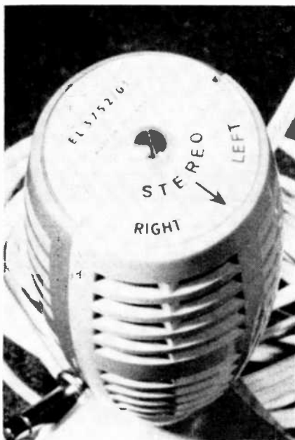
A stereo mike containing two separate mike cartridges is furnished with the unit. Arrow on top should be pointed toward middle of sound when a recording is made.
