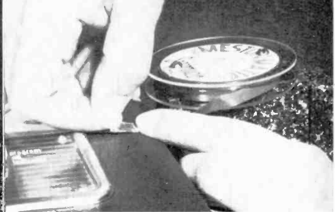
Upper left: after the unit is assembled, the synchronizer head is brought up to the level of the tape reel. The screw is then tightened to hold this position. Upper right: The tape runs from the head slot around the synchronizer head and back to the take-up reel. The synchronizer may also be placed so the tape is contacted before the head is reached. Lower left: showing how the tape is twisted as it leaves the head and again after leaving the synchronizer head. Lower right: applying the metallic tape tab.
