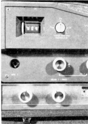
Right and left sides of the recorder face. Left side contains counter, speed change knob, channel 1 input jack and volume control and bass and treble controls. Right side of recorder has record/play lever, fast forward/rewind, edit key, VU meter, monitor switch and stereo monaural selector switch.
