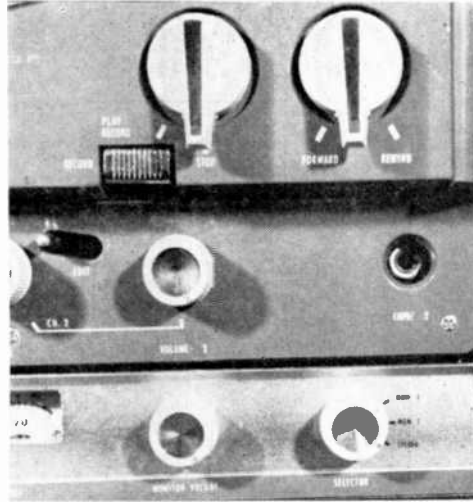
Right and left sides of the recorder face. Left side contains counter, speed change knob, channel 1 input jack and volume control and bass and treble controls. Right side of recorder has record/play lever, fast forward/rewind, edit key, VU meter, monitor switch and stereo monaural selector switch.
