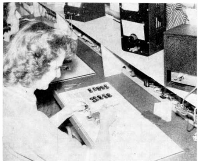
"For ladies only" might be the tag on this delicate job of inserting the super-thin foil in the head at one stage of the assembly.
