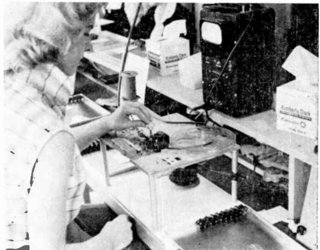
Before heads are packed for shipment they are tested on an actual tape deck using a tape loop to provide the signal, the results of which are indicated on the meter.
