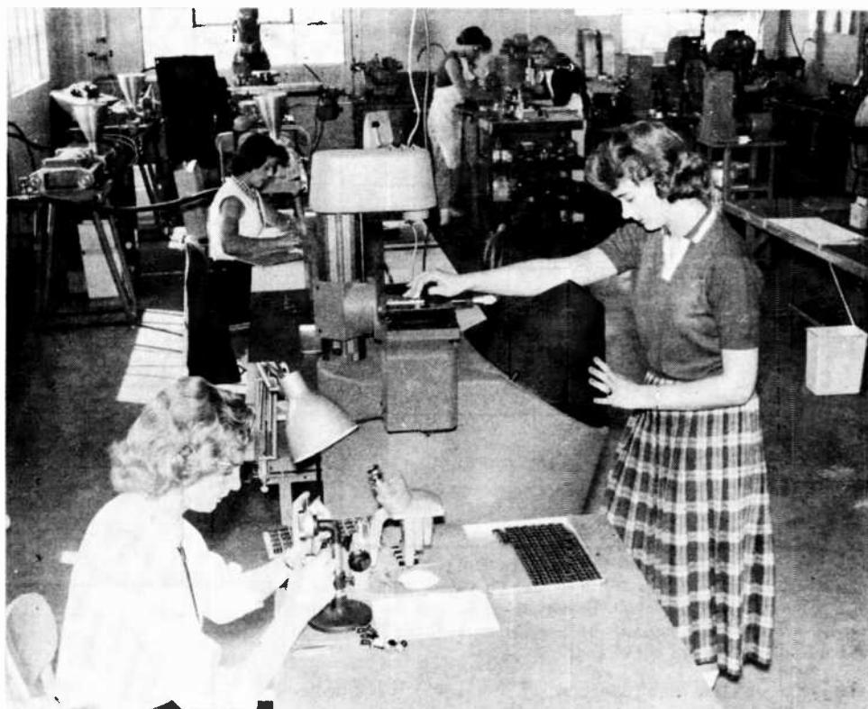
In addition to the electrical inspection, each head is subjected to a visual mechanical inspection on a device which presents a very greatly magnified image. The girl in the foreground uses a binocular microscope and a measuring gauge which indicates whether or not the heads are within the tolerance limits. All photos are from the Allegan plant of Michigan Magnetics.
