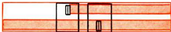
The Add-A-Track principle is shown above. The one part, accompaniment or otherwise is recorded on the lower track and picked up by the playback head at right. The new material is recorded on the other track by the top part of the head at left.
