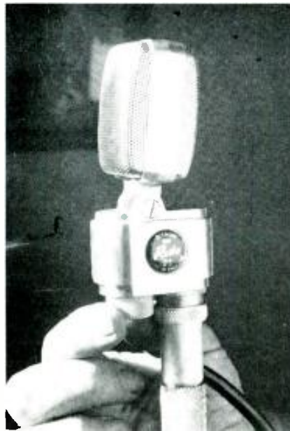
Above: the polar pattern characteristics of the mike may be altered by inserting felt and fabric pads as shown. These are placed in the back of the case. Right: the microphone may be had with or without switch. Knurled knob on bottom of case turns mike on and off.
