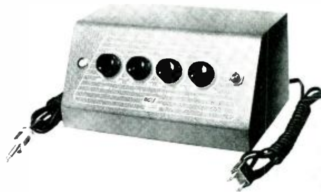
Masco model EMM-6 electronic mixer-pre-amplifier has six inputs (4 microphone and 2 phono). Three 12AX7 tubes, selenium rectifier. Cathode follower output—allows 400-foot separation from amplifier; any four channels are separately controlled.
