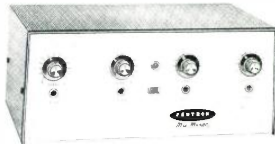
Pentron CA-14, 4-channel mixer with 6 high impedance inputs: 4 microphone, 2 phono (phono input receptacles are on rear of unit; microphone inputs are on front panel); provides 8 db gain in microphone channels. Tubes are 2—12AX7.
