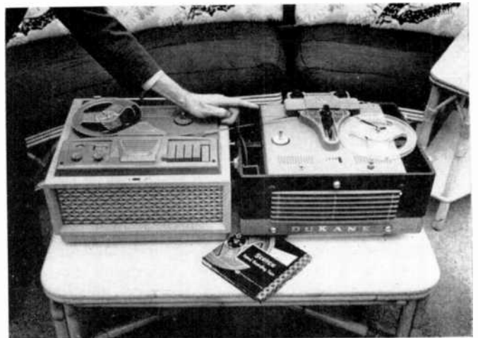
This shows how an Ampro and a DuKane recorder may be used for binaural recording. DuKane also has Shoup heads which may be inverted. A half twist in the tape is necessary with these machines.
