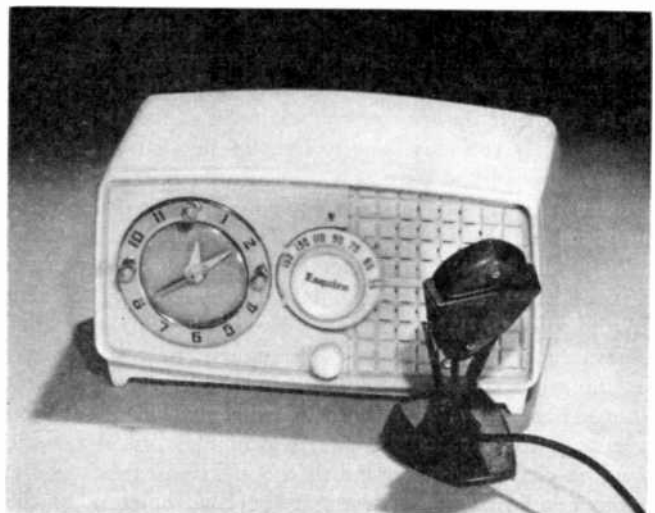
If you do not care to install a permanent plug, as shown on the next page, you may set the microphone in front of the speaker. In either case, run a test for recording level before leaving the house.
