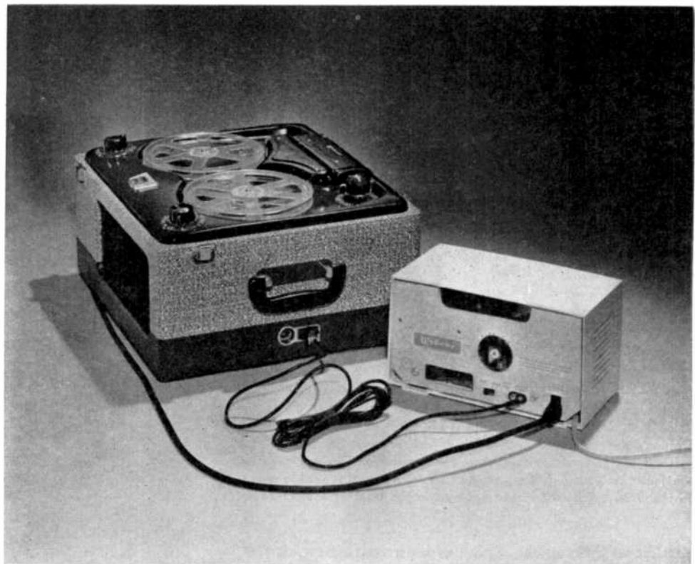
The rear of the Quintet clock radio showing the special receptacle into which the recorder input cord is plugged. The recorder line cord is also plugged into the appliance socket on the clock radio.
