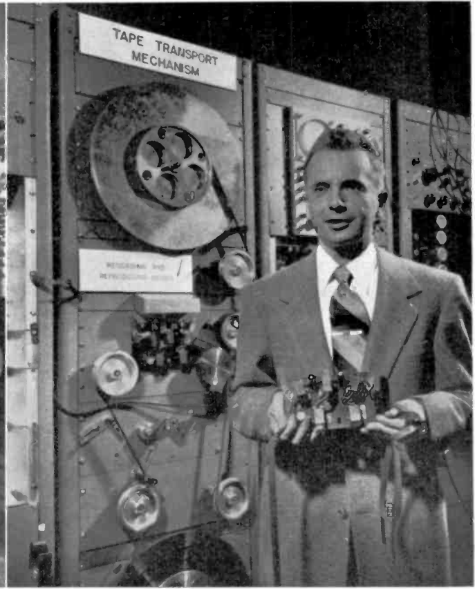
Joseph Zenel, research engineer, holds an experimental recording head unit, the heart of the video tape recorder. These heads have been specially designed to respond to the high frequencies used in TV which run out to 4,000,000 cycles per second as compared to the maximum audio range of about 20,000 cycles per second.
