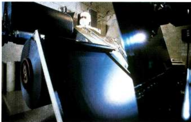
'Dry' end of tape coating line showing coated 'jumbo' rolls of tape
