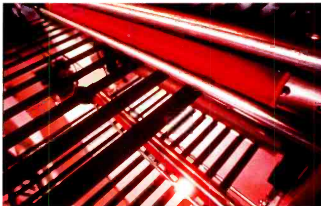
View of a tape slitter showing individual slit strands of tape
