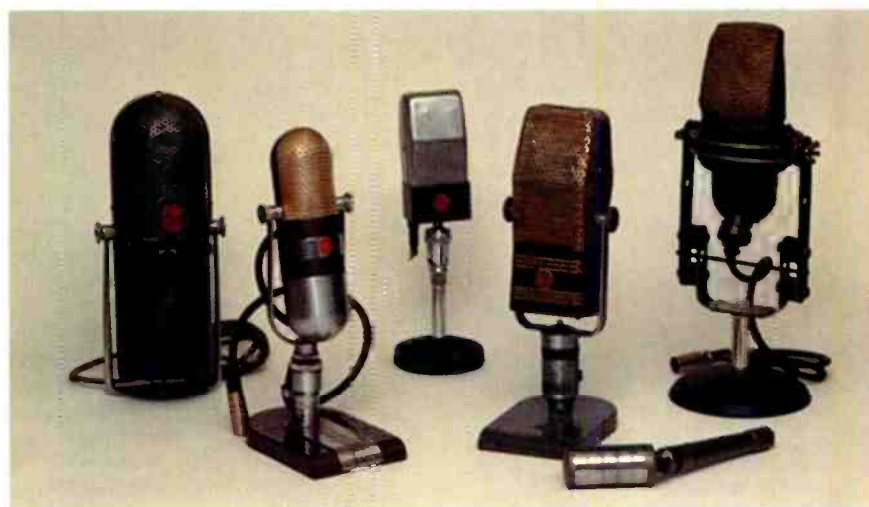
RCA ribbon mics including the model 77A from 1930
