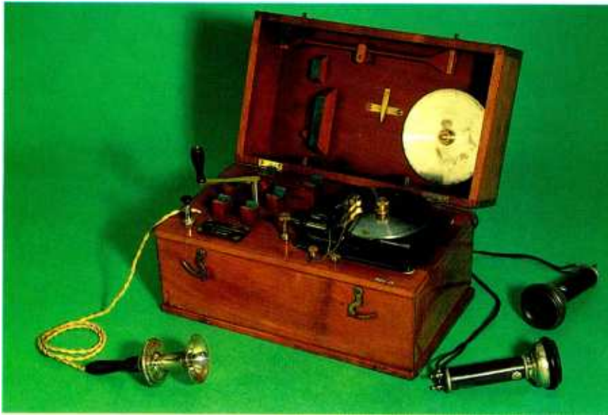
Clockwork disc-type Telegraphone for early recording and replay —as a Dictaphone, for example
