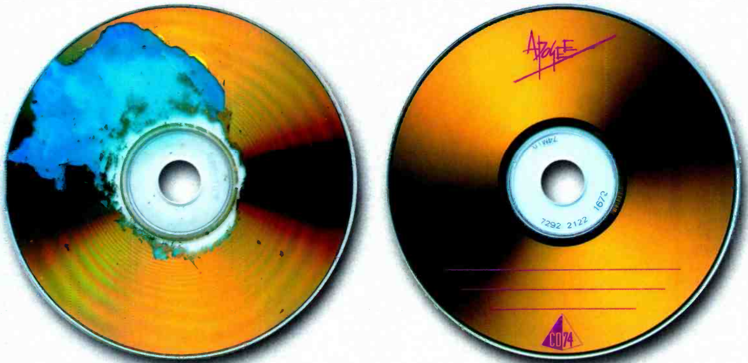
(Yes, they're real discs. The upper surface of each disc was cleaned for the same length of time with a lint-free cloth soaked in 91% isopropyl alcohol – a recommended cleaning technique for CD-R media. Ours, of course, is on the right.)
