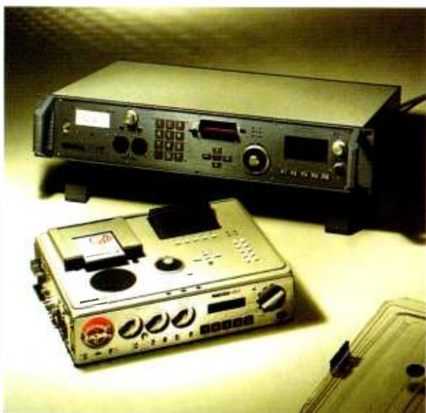
Nagra Ares-C—in-built ISDN codec, or SMPTE-EBU time code
