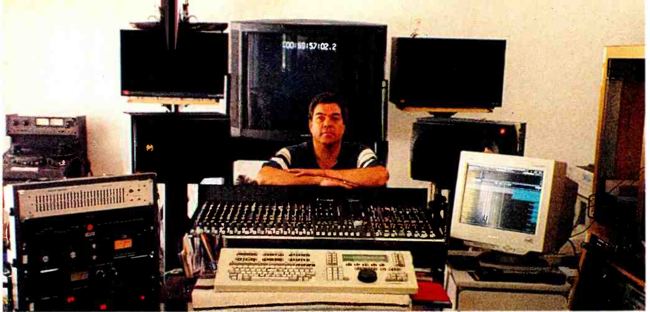
Albert Lord among his studio equipment: Sony XB12 Trinitron 35-inch TV; Soundcraft Ghost console; Fairlight MFX3 digital workstation; JBL 4412 and 6208 speaker systems; Urei bl-amp; Yamaha SPX90; MasterRoom reverb; Gain Brains; Sony SVP 5600 1/2-inch VHS deck
