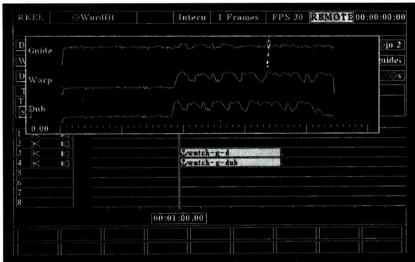
The SoundStation screen following WordFit processing. Note the three display plots: the Guide which is the original location voice sound; the Dub which is the replacement voice; and the Warp which is the WordFit processed Dub track
