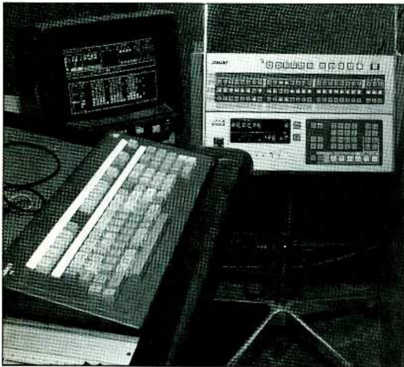
Adams-Smith AV2600 synchronisation system with the Sony autolocate
