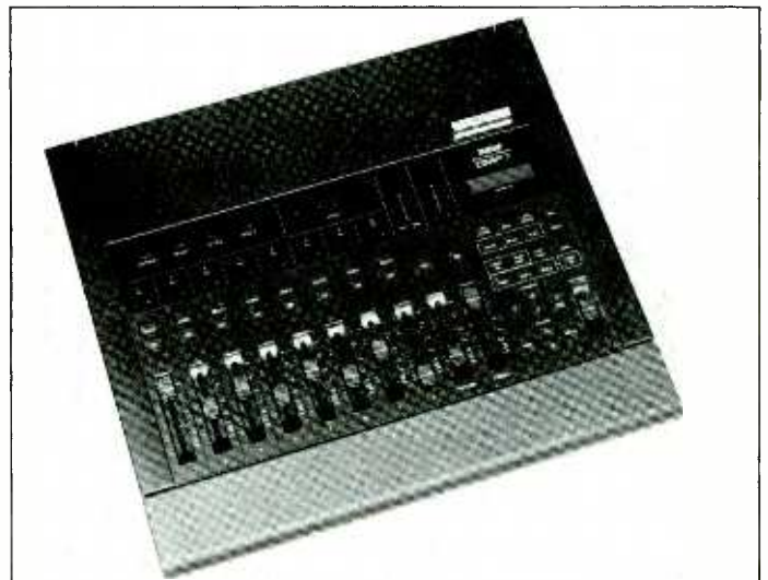
Yamaha's DMP7 incorporates effects and automation
