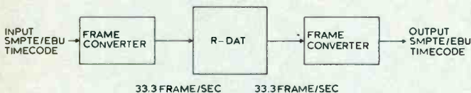
Frame conversion between SMPTE/EBU code and RDAT implied by a proposed standard
