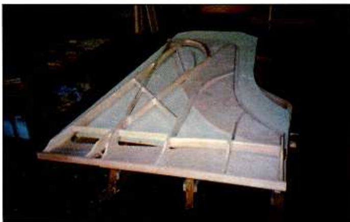
Construction of wooden template frame for new 3.8 m model
