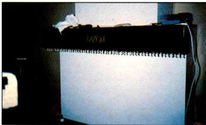
Unique machine for breaking-in pianos—it plays all notes at once till turned off
