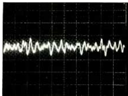
FIG. 13 CROSTALK AT 15 IN/S ZERO LEVEL -70dB
