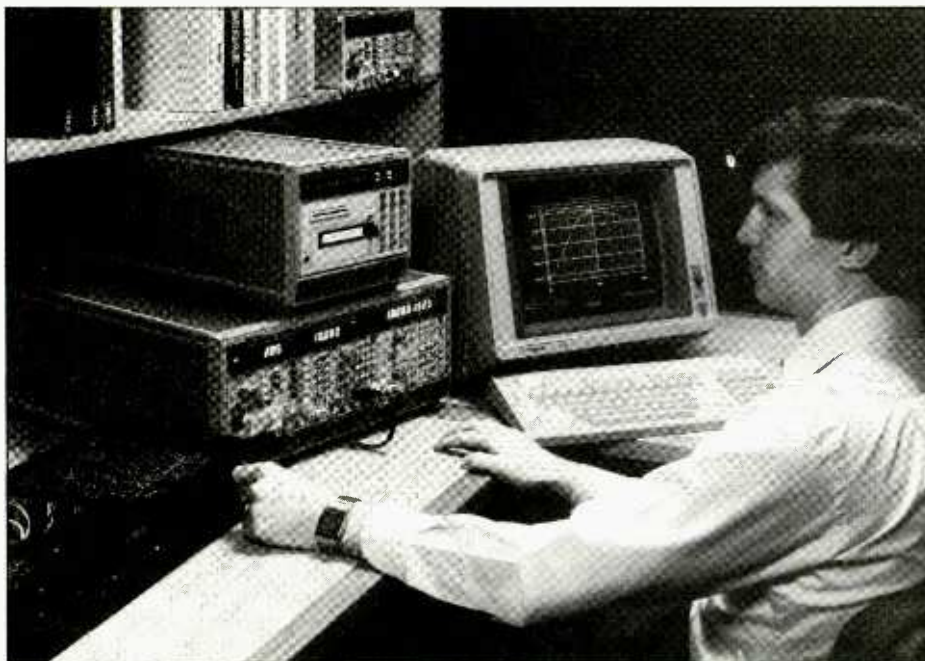
MP 2902 audio measuring package from Tektronix which includes the SG 5010 programmable oscillator
