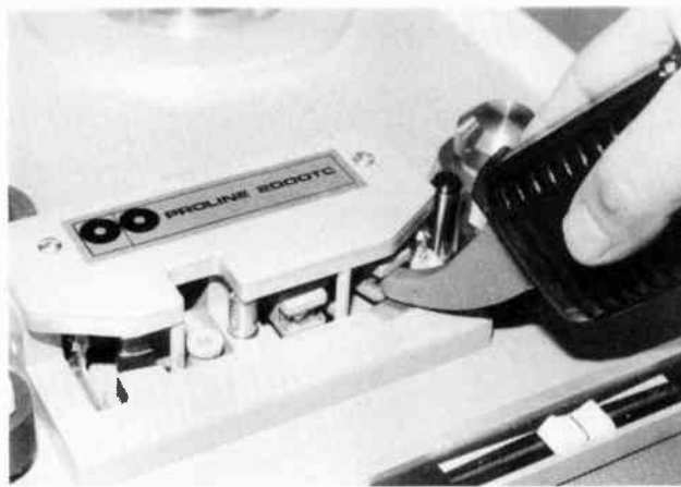
FIG.2 DEMAGNETISING A TAPE HEAD. NOTE THAT THE DEFLUXER SHOULD BE DRAWN STEADILY AWAY FROM THE HEAD BEFORE BEING SWITCHED OFF
