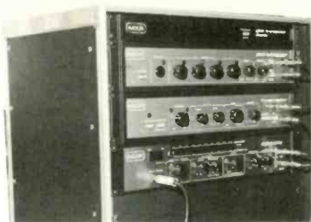
MXR digital delay, flanger/doubler and pitch transposer with optional display
