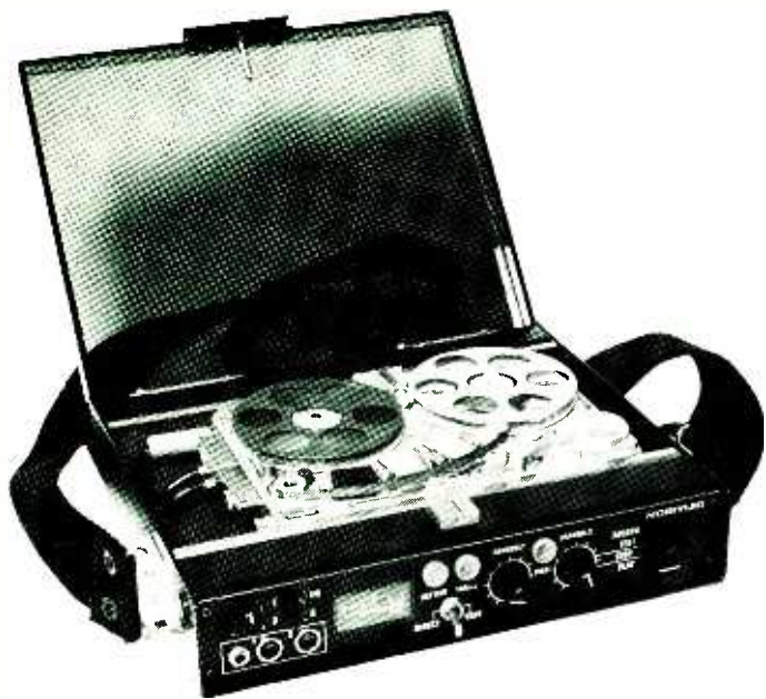
The Noriyuki SNM-3 minimixer and its raison d'etre, the Nagra SN. Front-panel controls include headphone gain; dynamic or a/b powered capacitor mic switch; 'flat' or low-frequency cut switch; battery check; 1k Hz tone button; 'direct' or 'off-tape' switch; gain controls for the two mic inputs; and a function switch. Price in the UK is about £650. A 'multiplier' unit will be available shortly to convert the 10 Hz pilot tone to 50 Hz (plus separating it from the audio signal). This will allow taped material to be transferred to a Nagra 4 machine, or facilitate direct dubbing in a 50 Hz transfer bay.
