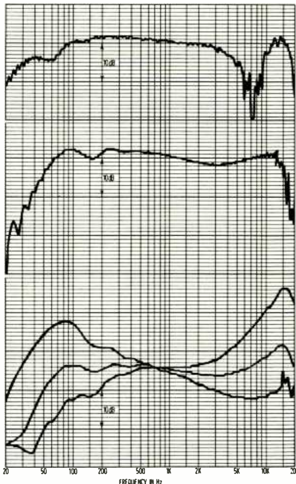
FIG. 2 DENON FREQUENCY RESPONSE REPLAY HEAD 4 FAST SPEED
