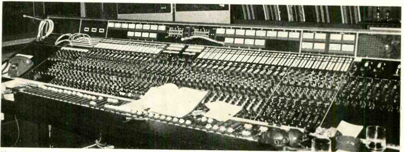
Hansa Tonstudio, Berlin. Sophisticated 32 channel quad console for 24 track recording.
