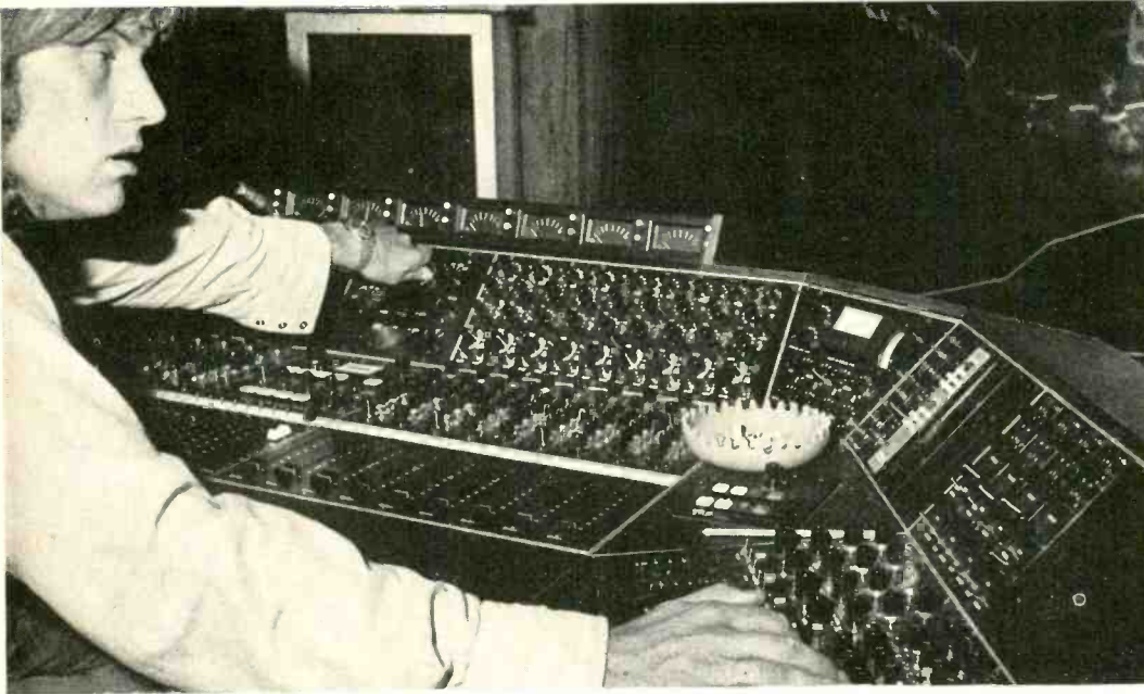
Alvin Lee Ltd. Ultra low profile console for 16 track recording in an elevated control room,
