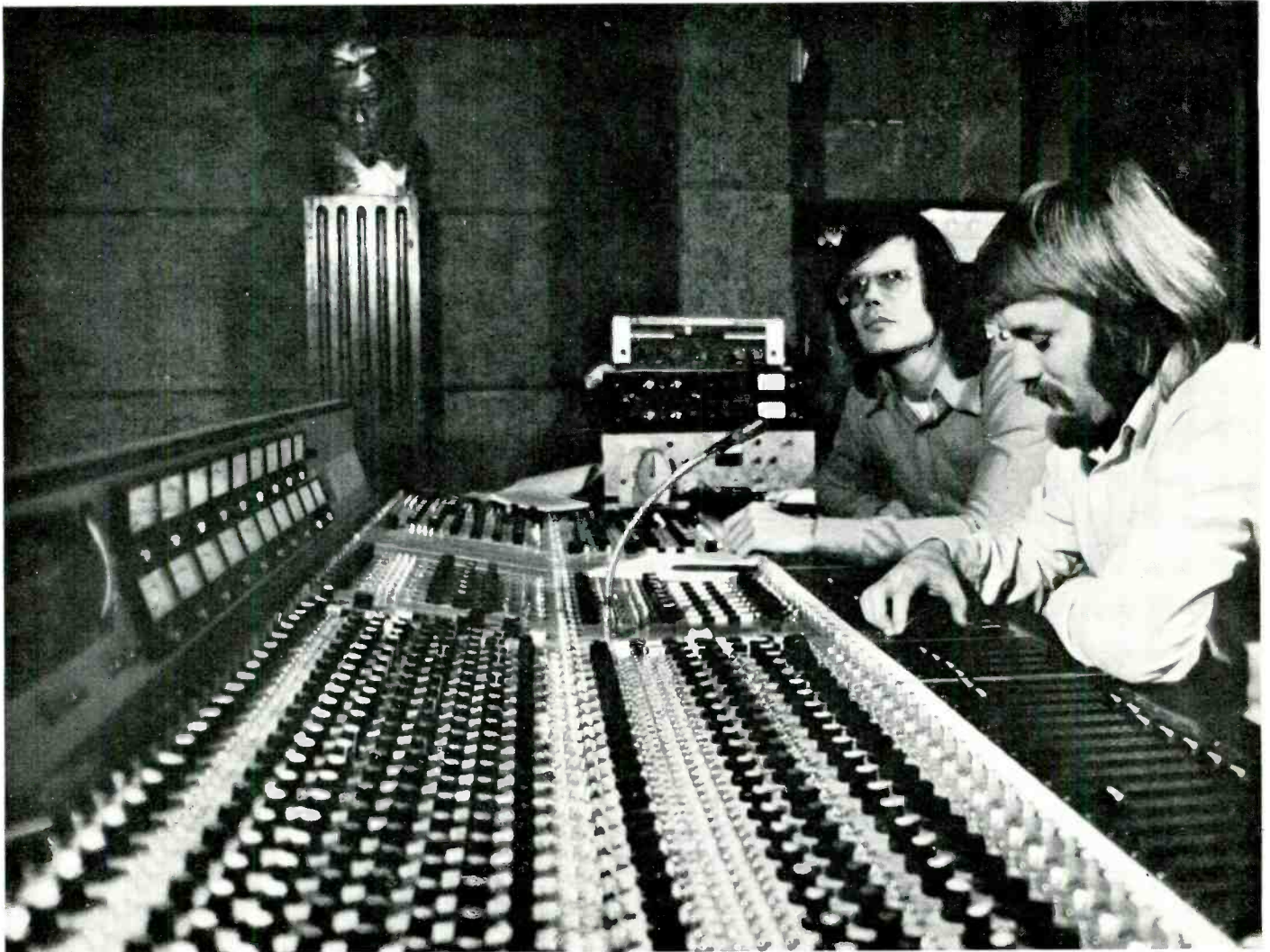
This console was supplied 32 into 8, wired for up-dating to 32 into 16 considering future studio expansion.
