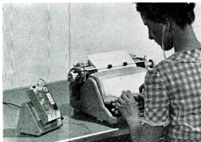
The Fi-Cord "at work" in the office. The foot control and stethophone headset assist the secretary to transcribe letters simply and efficiently.
