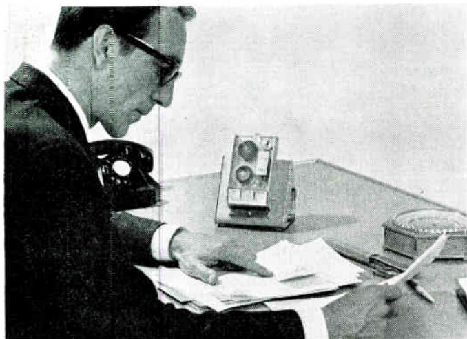
The built-in microphone permits the operator to continue working yet leaves both hands free.
