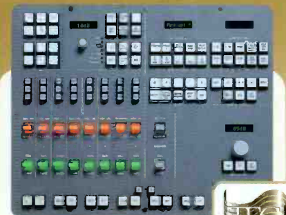
The 32:8 film scoring monitor section delivers the flexibility of printing a score to upwards of 16 tracks for final mixing at the dubbing stage.
