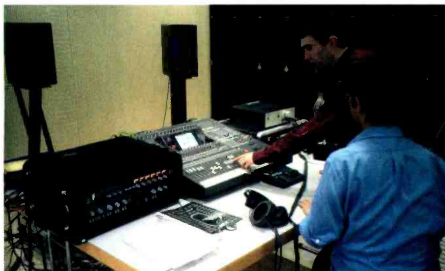
Sound Arts' Simon Fox and Koichiro Hattori (seated) at the Yamaha 02R with Soundfield SP451 and MkV controller to the left. Manger Zerobox 109 speakers in the background
